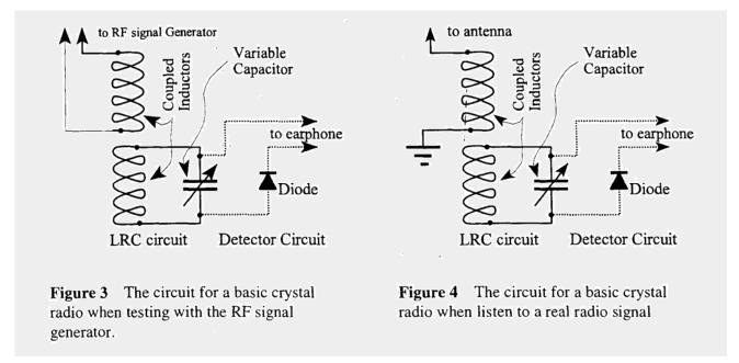
Assemble the circuit as shown in Fig. 3. Set the RF signal generator as suggested in the section on testing the signal generator. Set the capacitor box as calculated above. While listening, tune to get the loudest signal by varying the capacitance. Make a table to capacitances to tune various parts of the AM band (530- 1600 kHZ). Also note the range of capacitance that can tune an RF frequency.
